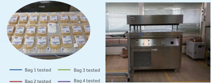
Core temperature of plasma reaches -30°C within 30mins
