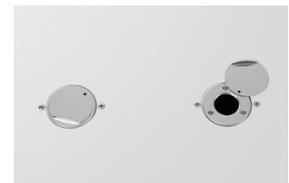
It is equipped with portholes to facilitate external equipment monitoring to record the experimental process.
