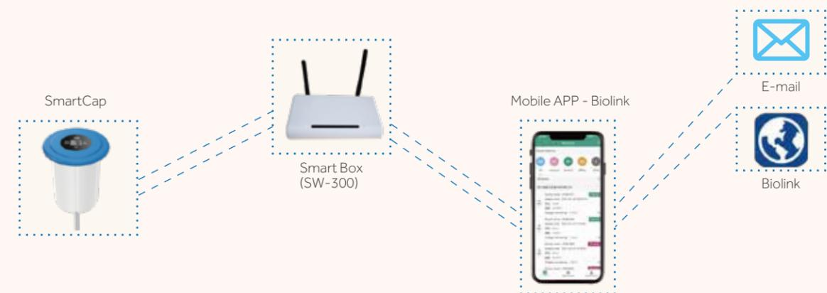
The SmartCap collects liquid level data and temperature data and transmits the information to cloud data store wirelessly, via 2.4G at a fixed interval every 10 minutes. Users can check real-time data and system alarm situation at any time through the Haier mobile APP-Biolink.
