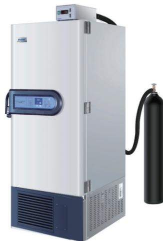
LN<sub>2</sub> backup cooling system is an independent refrigeration system for a ULT freezer. When there is a loss of power or the temperature of the freezer rises to the high alarm set point, the LN<sub>2</sub> backup system can be automatically activated to inject LN<sub>2</sub> into the chamber to maintain the freezer temperature. The backup system operates on a rechargeable battery when there is a loss of main power.
